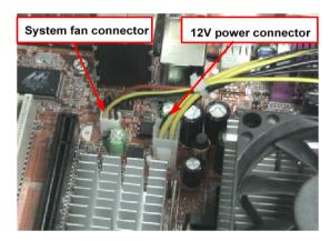
**4.** Disconnect the P1 power cable and ODD data cable from the main board connector.
